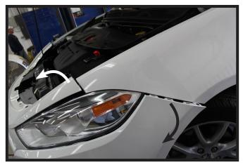
5. Pull edges of fascia up and out to separate from body. Repeat on other side of vehicle. Then remove the fascia from vehicle disconnecting any electrical connections and set aside.
