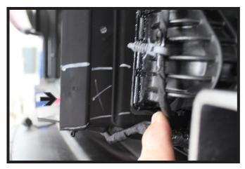
7. Trim the plastic shrouding in front of radiator on both sides of the vehicle approximately as shown for clearance of the baseplate installation. Further trimming may be required until baseplate clears the shroud.
