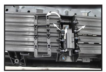
10. Remove the bracket in the middle of the shutter. Remove the second blade from the top of the shutter on both sides. Then reinstall the bracket.
