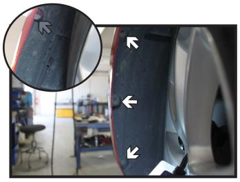
Using a 10MM socket, remove the one (1) upper screw from wheel well (inset). Using a 8MM socket remove the lower three (3) screws from wheel well (white). Do this on both sides of vehicle.
